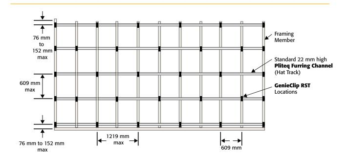
Wall or Ceiling Framing at 406 mm o.c. **GenieClip RST** at 1219 mm o.c., furring at 609 mm o.c. 1 or 2 Layers of 16 mm plasterboard
