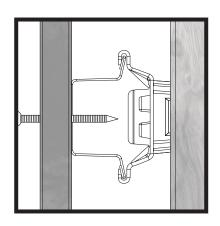
NOTE It is impossible to "short circuit" the **GenieClip RST**System when the correct screws are used. Should the installer hit a clip location, they will not be able to 'seat' the screw. They will be forced to move left or right on the track away from the **GenieClip RST**.
